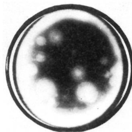
Figure 3. Chemical waves with aniline. For experimental conditions see Table I. Thickness of the layer: 0.07 cm.
